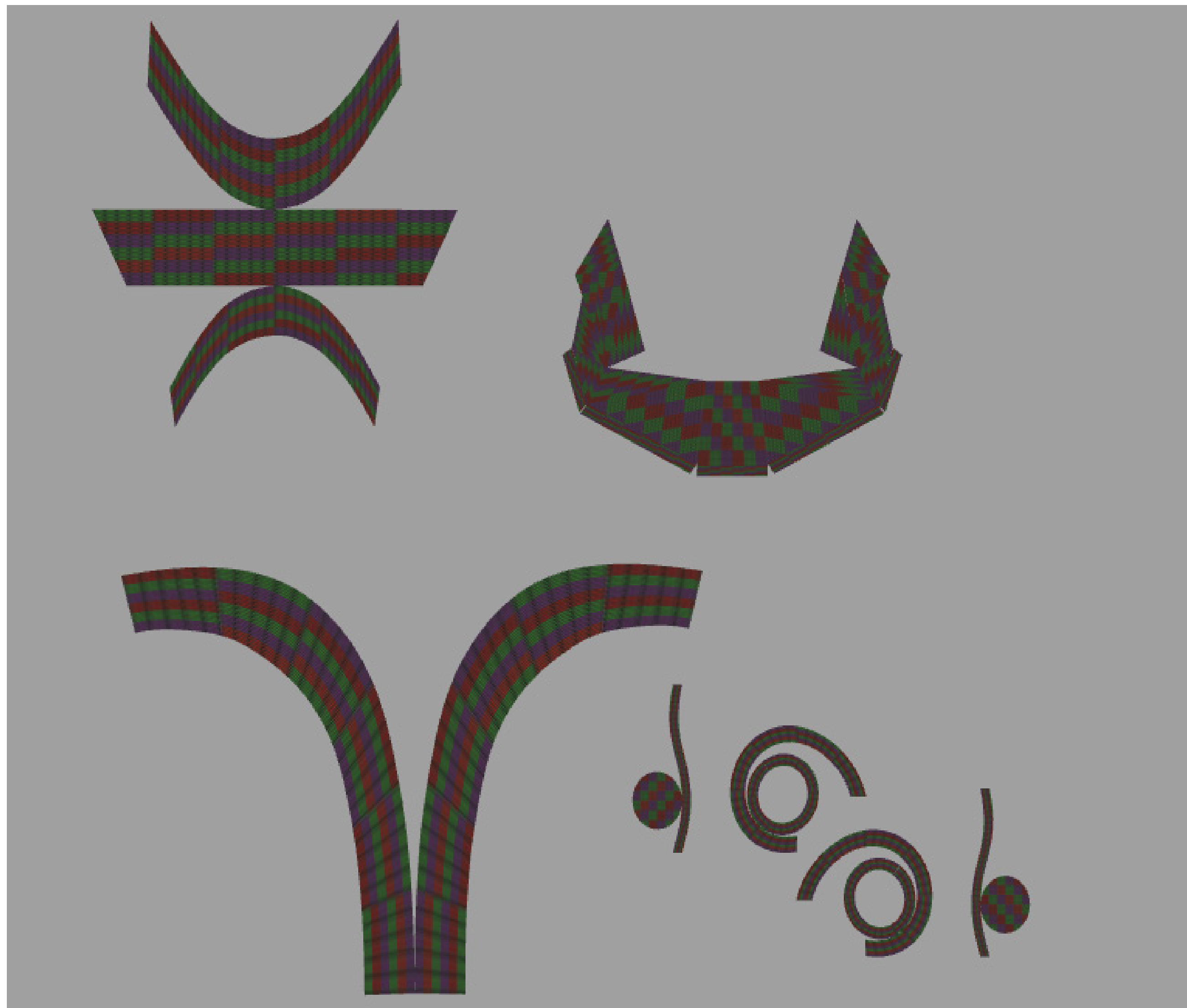
2D Unfolded Surface on Texture Map
